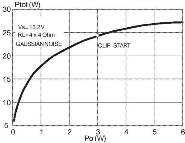
Figure 16. Power dissipation vs. output power (Music/Speech Simulation)
